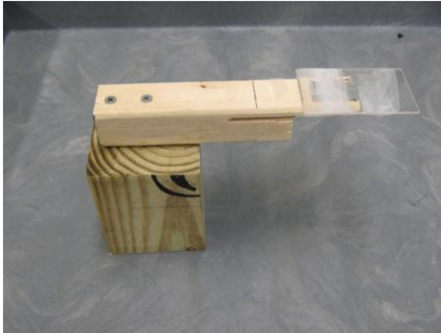
Figure 12: PsArs holder used to center positron source in 3\gamma/2\gamma , calibration, and efficiency experiments.
